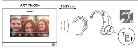
Make sure that the hearing aid is between 15 and 25 cm away from the monitor to ensure maximum audio quality during communication with the door panel.
