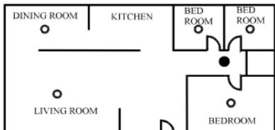
Figure 1: Installation locations for smoke & heat detectors in single-family apartments or homes with only one sleeping area
