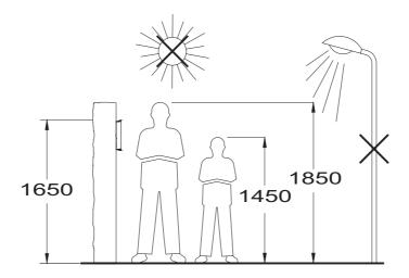
Locate the top of the door panel at a height of 1.65m.
