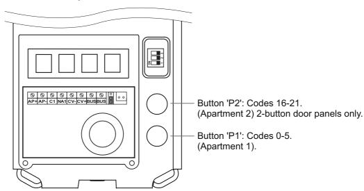
The sound module's P1 and P2 buttons are assigned with factory codes.
