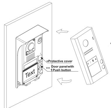
To finish the mounting of the door panel, replace the metal front.
