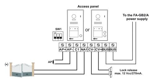
(\*) - To switch voltages higher than 12Vdc/1A between terminals 'C1' and 'NA1' on the door panel, consult our technical service department. - 'C1' and 'NA1' potential-free contact.
