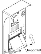
After completing the wiring and configuration work, position the nameplate label in the electronic module. Fix using the screws supplied.
