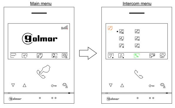
To make an internal intercom call (to another monitor(s) in the same apartment), press the buttons below corresponding icons  $\nabla / \triangle$  to select the monitor to be called, press the push button below the icon  $\sqrt{}$  to make the call. Note: The selection .: Not use with KIT S5110 ART4W LITE.
