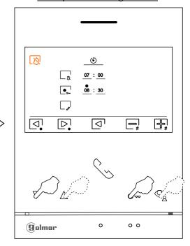
Press the push button below the first icon to return to the main menu screen. If the "automatic door opening" mode has been activated (see page 23) the right icon will be displayed at the top left of the main menu screen and the led of the rush button will blink in white color when the monitor is in standby mode (screen off).
