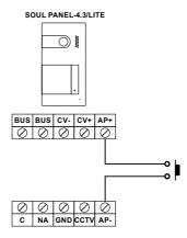
IMPORTANT: Installation with 2 access door panels and AP button on both door panels, one of the door panels must connect the AC lock release (instead of DC lock release) with a SAR-12/24 relay and a transformer TF-104, (see pages 26, 27 and 28).
