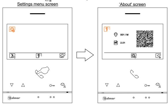
To restore the monitor to factory settings, press the button below icon to access the factory reset menu, then press the button below icon to perform this function. Press the button below icon to return to the 'About' screen.
