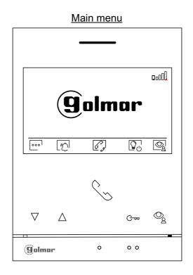
If the device is in standby (screen switched off), to access the main menu, press any of the buttons of the monitor. Then press the button located just below the corresponding icon. The device will return to standby mode after 20 seconds without activity.
