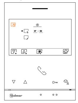
To set a period of time for "Do not disturb" mode in which the monitor will not sound when receiving 00h & 01 minute to 23h & 59 minutes) for 'Do not disturb' mode, by pressing corresponding buttons 4 / A and 4, validate the changes made by pressing the button below icon 4.
