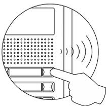
Make a call to check that the monitor has been successfully programmed. Programme the other monitors in the same way. Once the programming has finished, set the programming switch to OFF. If this is not done, the door panel will emit tones to indicate that the system is still in programming mode.
