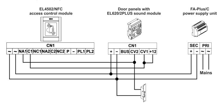
Audio door entry systems with one access door and 4+"n" installation.
