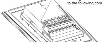
The wiring terminals are located at the back of the module and correspond to the following connections:
