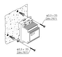
Install the transformer in a dry and protected location.
