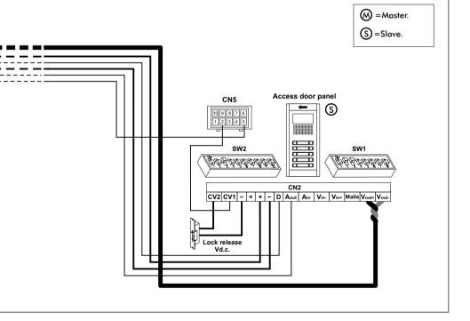
Video installation with coaxial cable and 2 switch units.
