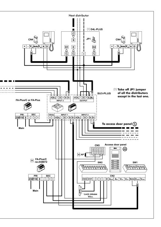
Video installation without coaxial cable and 2 switch units.
