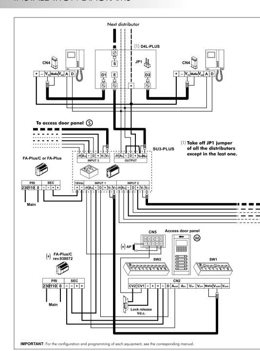
Video installation with coaxial cable and 1 switch unit.
