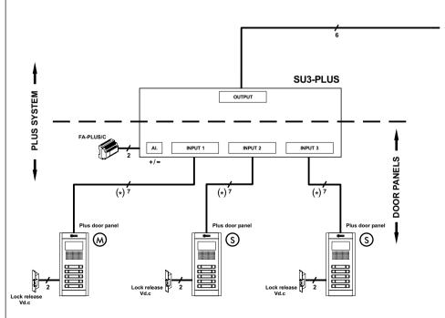
(\*) Door panel without power supply needs 7 wires (to connect the '+' terminal).
