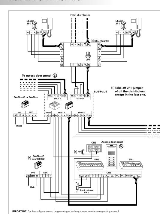
Video installation without coaxial cable and 1 switch unit.
