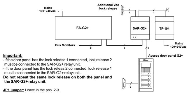
(\*) The power supply of the lock release is connected in series through the SAR-G2+ relay contacts.
