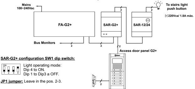
(\*) Neutral point of the power supply of the stairs light is connected in series through the relay contacts of the SAR-12/24. **IMPORTANT:** For the description, installation, configuration and programming of the system, see the corresponding manual.
