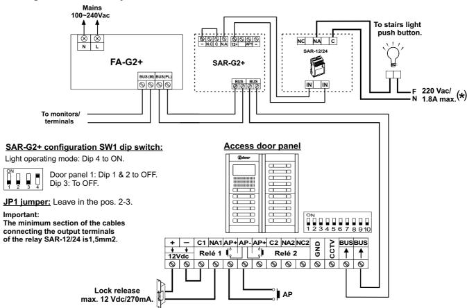
(\*) Neutral point of the power supply of the stairs light is connected in series through the relay contacts of the SAR-12/24.
