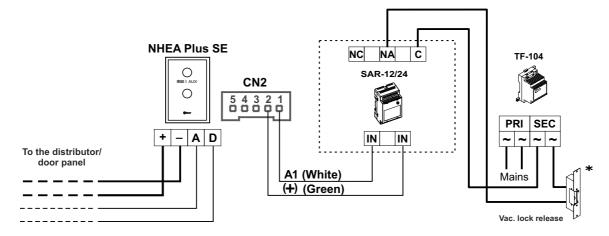
\* **Important:** Place the varistor supplied with the sound module directly onto the terminals of the lock release.
