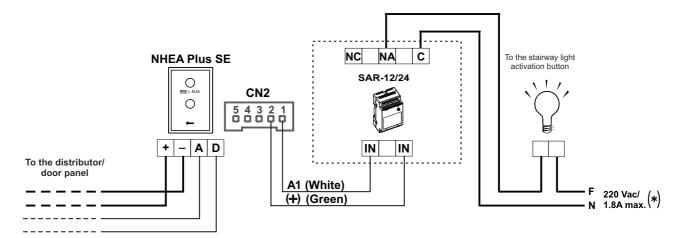
(\*) The neutral of the lighting power supply is arranged serially through the contacts of the SAR-12/24 relay and the maximum consumption of the element to be connected does not exceed 1.8A.
