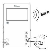
3. Go to the monitor/telephone of apartment B that has to call the button to be programmed in <u>Step 2</u> and press the door release button. The monitors/telephones emit a completed programming beep.
