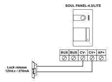
If the lock release to be used is alternating current, use a relay and transformer suitable for the consumption, as well as the varistor supplied. The example shows a Golmar SAR-12/24 relay and a TF-104 transformer (12Vac/1.5A).
