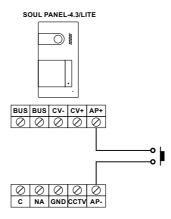
IMPORTANT: Installation with 2 access door panels and AP button on both door panels, one of the door panels must connect the AC lock release (instead of DC lock release) with a SAR-12/24 relay and a transformer TF-104, (see pages 24, 25 and 26).
