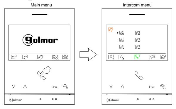
To make an internal intercom call (to another monitor(s) in the same apartment), press the buttons below corresponding icons ♥️/♠ to select the monitor to be called, press the push button below the icon ♥ to make the call. Note: The selection ♥ Not use with KIT S5110 ART4 LITE.
