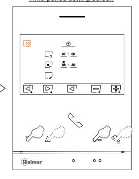
Press the push button below the first icon to return to the main menu screen. If the "automatic door opening" mode has been activated (see page 21) the real icon will be displayed at the top left of the main menu screen and the led of the real push button will blink in white color when the monitor is in standby mode (screen off).
