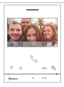
This screen is displayed when receiving a call or pressing the button below icon of the main menu. During a call, icon of the screen is in green color (during the call process). In the top left of the screen, the source of the image is displayed. The call has a duration of 45 seconds.
