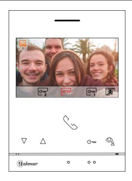
This screen is displayed during a communication process. During a communication, icon displayed on the screen is in green color. In the top left of the screen, the source of the image is displayed. The communication has a duration of 90 seconds.
