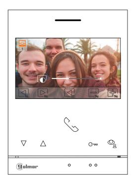
The following colour control menu will then be displayed. Adjust to the desired level by pressing the buttons below icons [-]/[-]. To access the monitor call tone / communication volume control, press the button below icon [-]. To exit the image and communication settings menu, press the button below icon [-].
