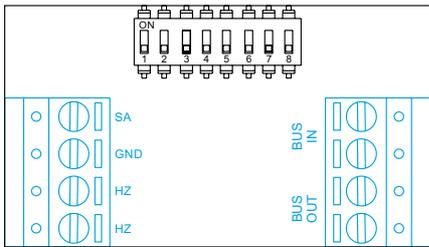
BUS IN: Communication bus input to monitor (non-polarised).
