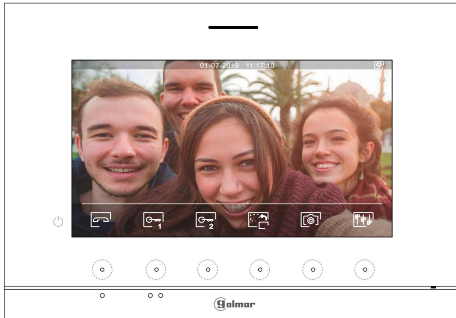
This screen is displayed during a communication process. In the top centre of the screen, the date and time are shown and, on the right, the source of the image is displayed.
