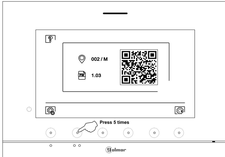
The 'special codes' screen will then be displayed. Press the hidden buttons below icons  $\nabla$  /  $\triangle$  to select the field to be modified and press the hidden buttons below icons  $+$  /  $=$  to enter the desired code. Once the code has been entered, press the hidden button below icon  $\checkmark$  to validate it. If the code entered is valid, icon  $\checkmark$  will be displayed; if it is not, icon  $\times$  will be shown.
