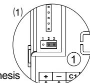
(1) Jumper placed between 2 and 3, set to minimum volume the vocal synthesis and tones from the door panel.
