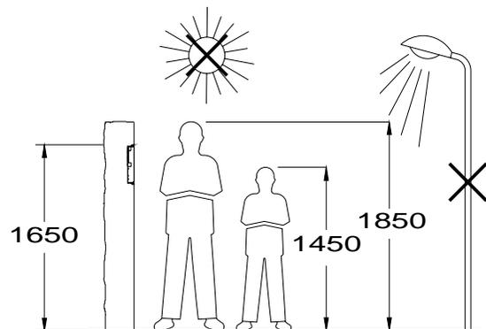
The upper part of the door panel should be placed at 1,65m. height roughly.
