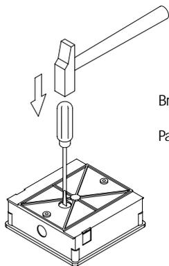
Break the bottom flange to pass the cables through.
