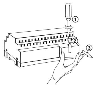
When the installation and wiring works are finished, place the protection cover before replacing the electrical current.
