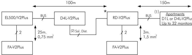
(2) Up to 1 RD-V2Plus for each distributed output of D1L or D4L-V2Plus distributor.
