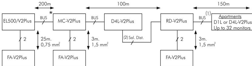
(2) Up to 1 RD-V2Plus for each distributed output of D1L or D4L-V2Plus distributor.
