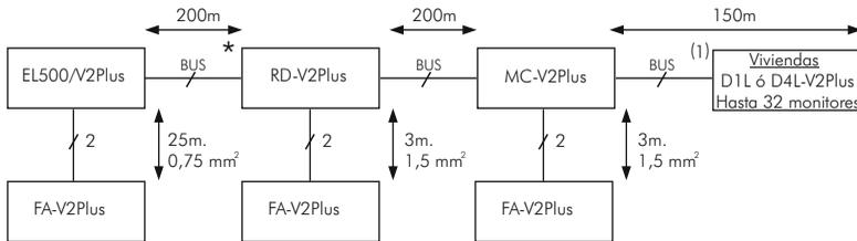
**C: 64 elementos por columna (500 metros):**
