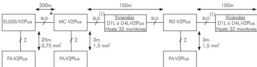
**D: Repetidor en cascada (32 elementos por columna / 600 metros):**
