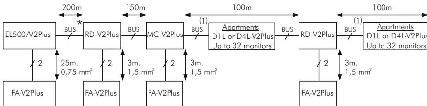
(1) **Important:** Do not exceed the max. monitors/telephones connected to a door panel/multiplexer/repeater, or the distances indicated for door panel/multiplexer/repeater and last monitor and monitors between different apartments connected to door panel/multiplexer/repeater. For characteristics, sections and distances see the corresponding product manual.
