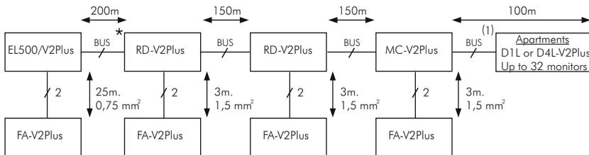
**F: Repeater in daisy chain (32 elements for riser / 600 meters):**
