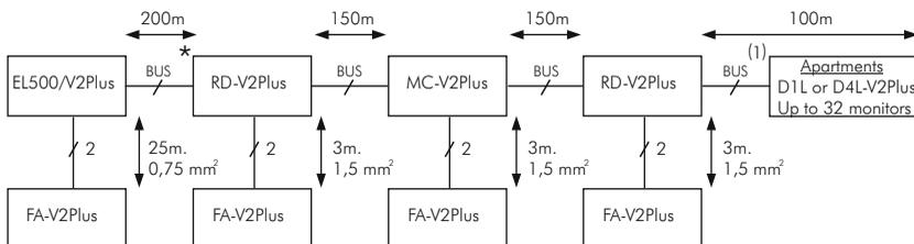
**G: Repeater in daisy chain (64 elements for riser / 550 meters):**
