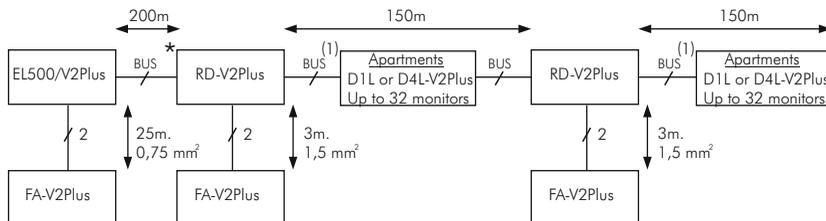
(1) **Important:** Do not exceed the max. monitors/telephones connected to a door panel/multiplexer/repeater, or the distances indicated for door panel/multiplexer/repeater and last monitor and monitors between different apartments connected to door panel/multiplexer/repeater. For characteristics, sections and distances see the corresponding product manual.
